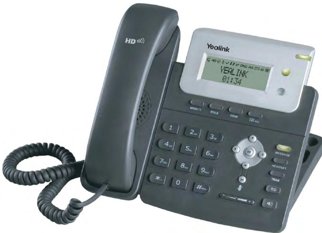
Yealink expands its lineup of IP phones with a new entry-level product SIP-T20P. It is equipped with TI TITAN chipset and 2x15 characters LCD, offers 2 VoIP accounts, high-definition voice, broad range of voice codecs, security protection for privacy, rich features including headset, PoE, PnP Auto-provision, and seamlessly work with the leading IP-PBX and soft switch.
